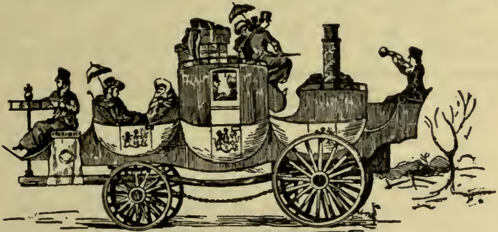
FIG. 10.—James' Coach (1829), the "first really practical steam carriage built." Drawn from an old wood cut.
